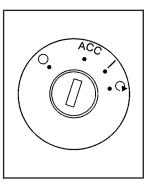
With the key in the ignition switch, you can turn it to four different positions. A warning tone will sound if you open the driver's door when the key has not been removed from the ignition.
